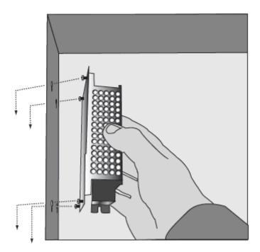
b. From the outside of the cabinet, tighten the screws to lock the power supply in place.
